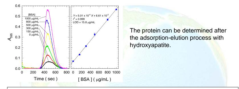
The pH adjustment is important for the effective adsorption-elution. The dilution with 10 mM buffer is required to adjust pH value for the artificial urine.
