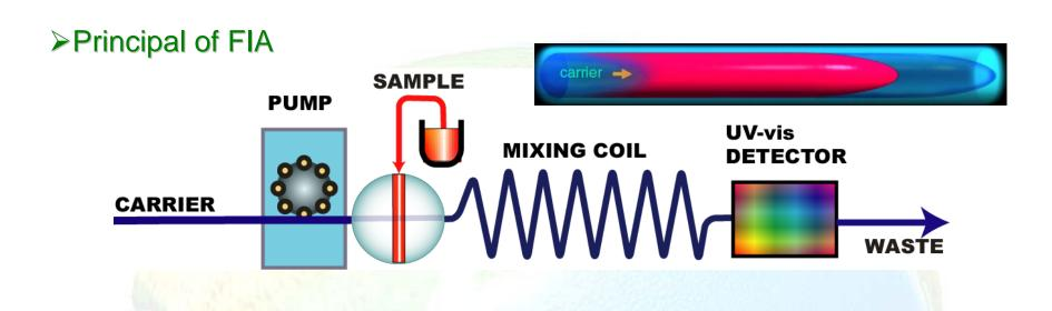
Liquid sample and reagent are added to the system, allowing the sample/reagent to be mixed and reacted.
