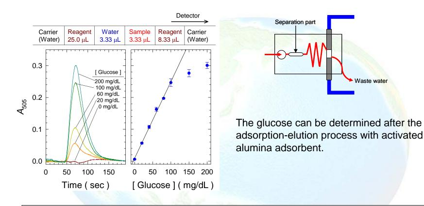
When the artificial urine ([Glu] = 80 mg/dL) was applied, 85.3 mg/dL of glucose was determined.
