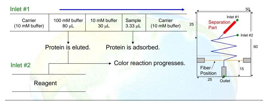
Two inlets, for sample and reagent stream, were used since hydroxyapatite was dissolved by acidic reagent solution.
