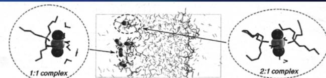
**Figure 3.** Enlargement of UO<sub>2</sub>(NO<sub>3</sub>)<sub>2</sub>·TBP·H<sub>2</sub>O and UO<sub>2</sub>(NO<sub>3</sub>)<sub>2</sub>·TBP<sub>2</sub> complexes that formed at the interface between water and SC-CO<sub>2</sub> upon demixing of system A.
